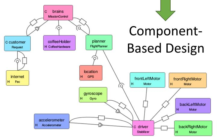
Diagram courtesy https://docs.sel4.systems/projects/camkes/visual-camkes/VisualCAmkES\_Layout\_Example.png • Components encapsulate and isolate state and functionality
